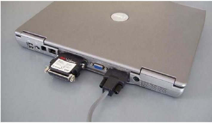
**Note:** Make sure the Enhanced FLASHKey is attached to the Parallel Port (USB Port if USB Dongle is being used) of the Computer.
