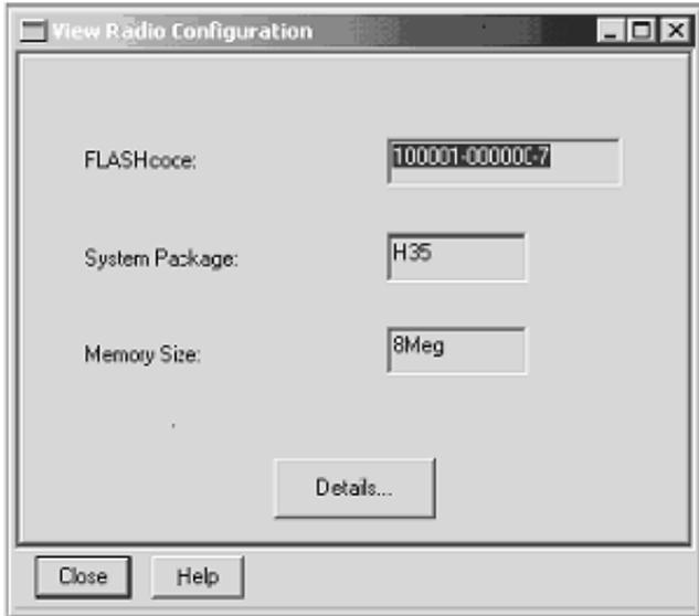
7. Close the *View Radio Configuration* screen. From the menu bar in the CPS main window, select:
