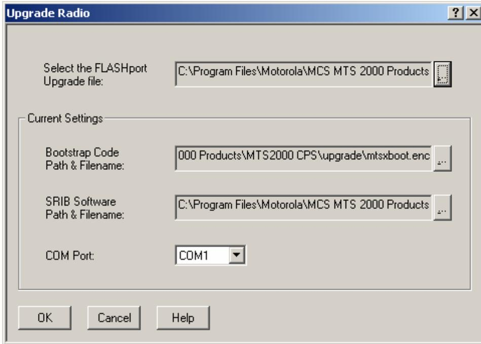
**Note:** Make sure the CVN or TVN file supplied on the CD with your FLASH Kit is located in the UPGRADE file of the CPS being used,
